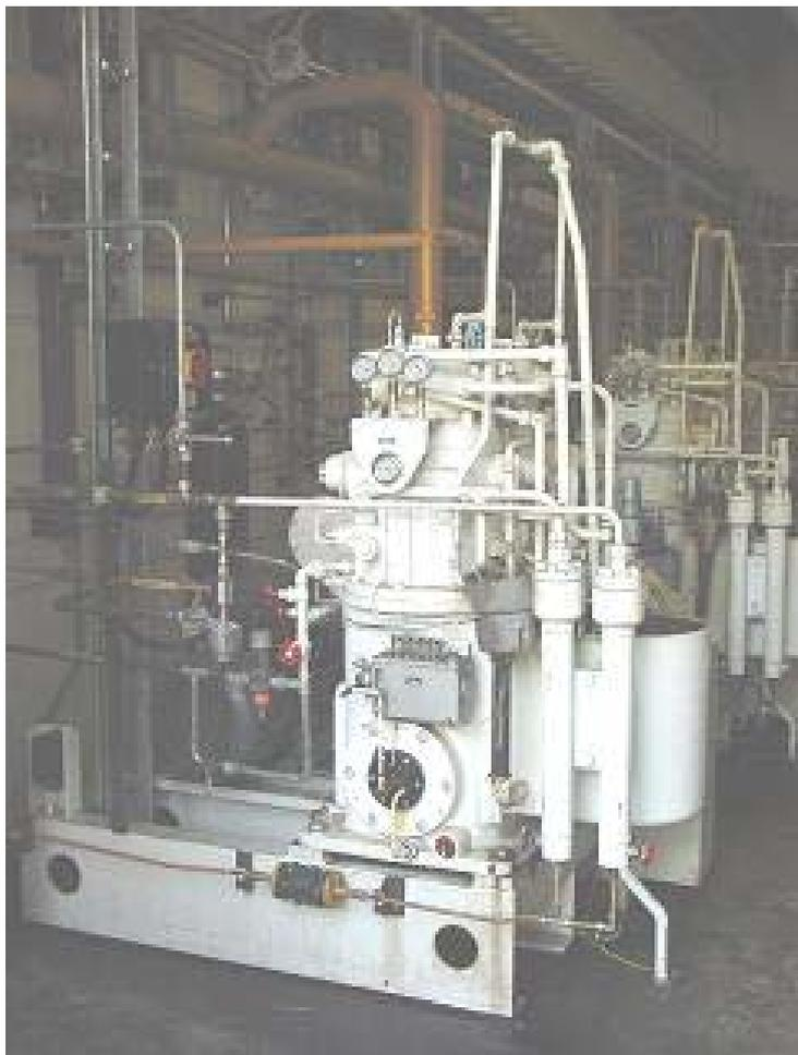
**Assumptions:** The compressor is installed in the high pressure building of the acetylene plant where acetylene cylinders are filled. The electric motor is located in a separate room which is not an ex-classified room and the axle between motor and belt pulley is going through the wall and is gas tight sealed. The compressor is belt driven. All safety valves at the compressor are piped above roof at a safe place. The outlet pressure of the compressor is 25 bar. It is water cooled.
