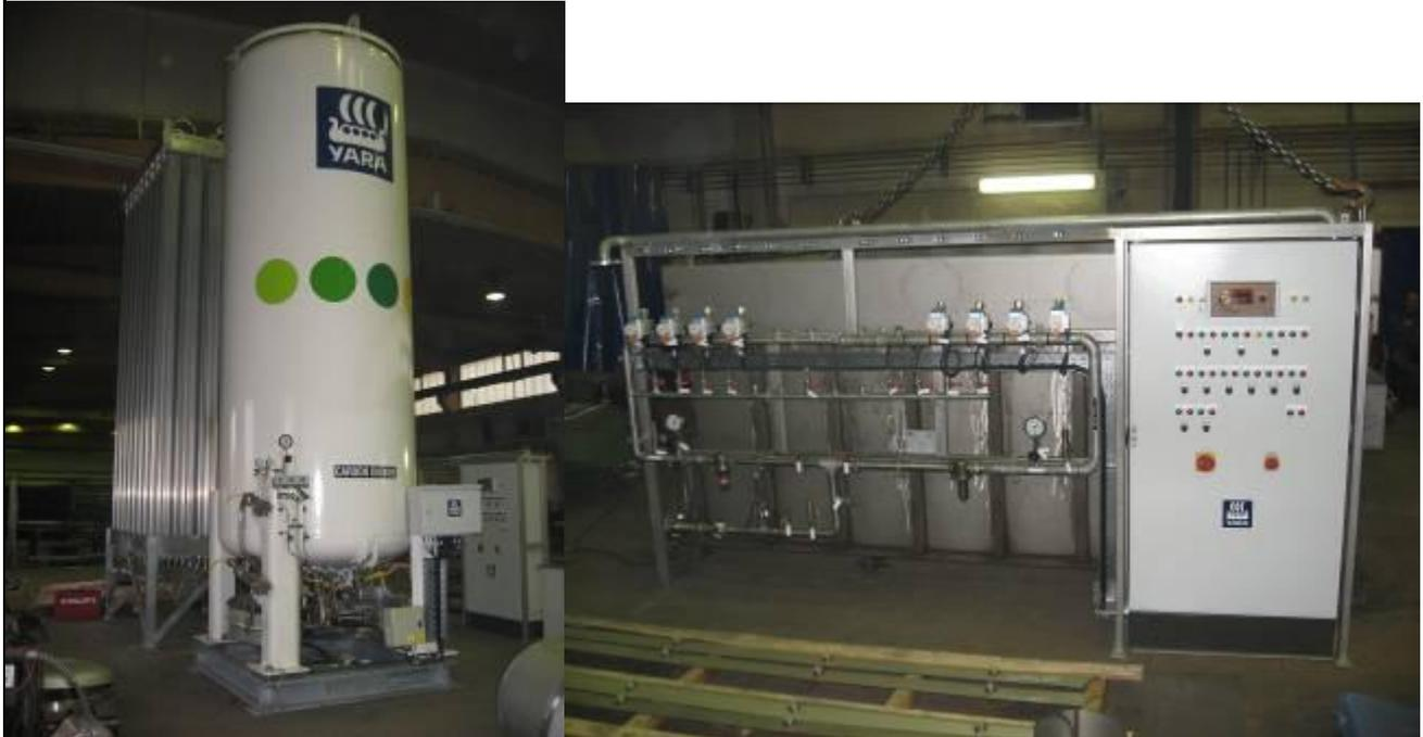
Combines advantages of controlled storage in combination with newest technology. These inerting systems are mainly used in countries with constant temperatures above +5° C and higher like Asia, Near East, Africa, Central and South America or Australia. Inert gas capacity is mainly depending on size of evaporizer and ambient temperature.
